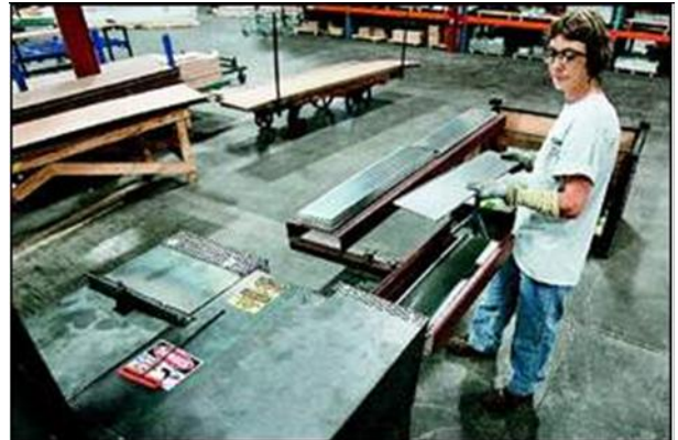
Employee Debbie Ashauer removes a finished piece of flashing from a roll forming machine at Appleton Supply Co. in Appleton last week. Post-Crescent photo by Kirk Wagner
